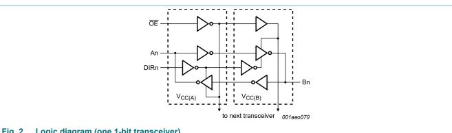
Fig. 2. Logic diagram (one 1-bit transceiver)
