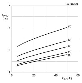
c. LOW to HIGH propagation delay (A to B);  $V_{CC(A)} = 2.5 \text{ V}$ d. HIGH to LOW propagation delay (A to B);  $V_{CC(A)} = 2.5 \text{ V}$
