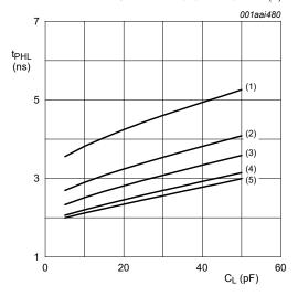
c. LOW to HIGH propagation delay (A to B); V<sub>CC(A)</sub> = 1.5 V d. HIGH to LOW propagation delay (A to B);  $V_{CC(A)} = 1.5 \text{ V}$
