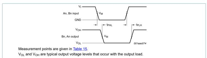
Fig. 4. The data input (An, Bn) to output (Bn, An) propagation delay times
